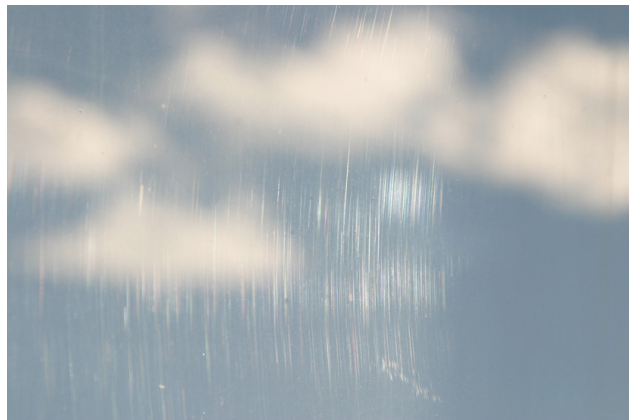
Figure 8: Another example of a window glass surface where the observed scratches are indicative of cleaning in the absence of an experienced professional.
